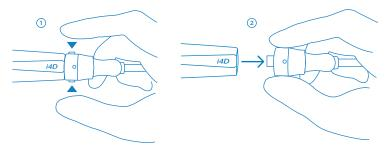
To reduce future wear and tear, press the two buttons when connecting the USB cable as well.
